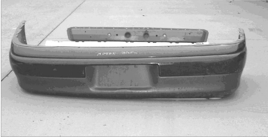
Figure 1. – Bumper cover with superficial damage.
