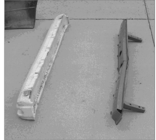
Figure 2. – Bent bumper reinforcement.
